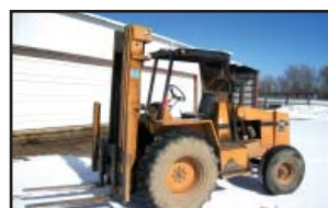
Conrac 706E All terrain forklift 18' lift
